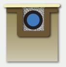
Sandtrapper II, MD and I are all able to be placed over drainage lines. By doing so, maximum performance against drainage gravel contamination is acheived.
