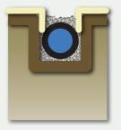
Should access be required to the drainage system, Sandtrapper can be tucked down and into the drainage trench.
